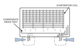
Remote pumps have the selection challenge of switch activation. Some pump designs use a seperate reservoir for mounting inslde the mini-split with an internal float mechanism and electronic switch. which activates the pump and can also disable the mini-split system during an overflow incident Other pump designs use a temperaturedifferential sensor switch that can be attached to the lineset to control pump operation.
